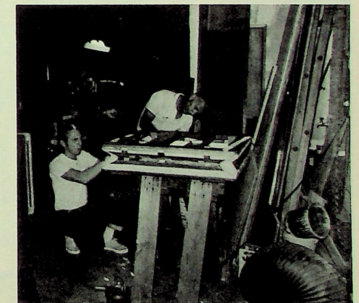
Roy Casavant and Dave Allard are shown at work re-leathering one of the large reservoirs of the Wurlitzer in the shop behind the auditorium building. All leather work in the instrument was replaced if it showed signs of wear. The reservoirs in a theatre organ are under high fluctuating pressure when in operation.
