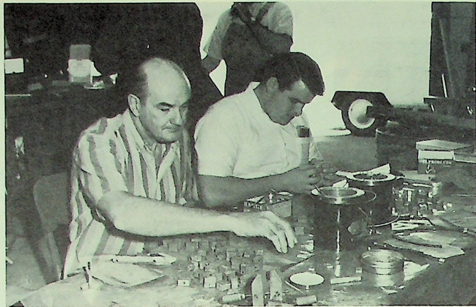
Hundreds of man hours went into the re-leathering of the Wurlitzer. Here Robert Brower and Ken Petersen are recovering hundreds of small pouches in the warehouse building behind the Auditorium. The job they are doing in the photo above was representative of the exacting and tedious but most necessary work for flawless operation of the organ.
