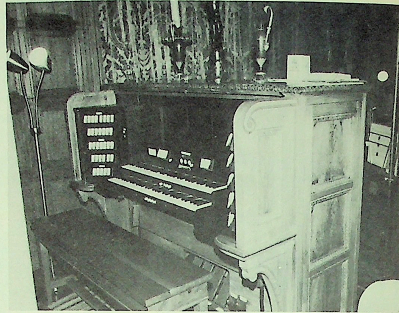
Console of the Lloyd two-manual, thirty-two rank Aeolian Duo-Art organ. Player unit is hidden by panels above the console backboard where music rack is normally found.
