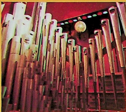
Foundation chamber front to back - English Post Horn, Tibia Clausa (large scale), Diaphonic Diapason, Tuba Mirabilis, Solo String, Tuba Mirabilis offset.
