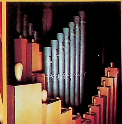
Wood pipes in background - 5 1/3' Gross Quint; Center - 8' extension of 16' Open Diapason; foreground - 8' extension of 16' Tibia Clausa (small scale).
