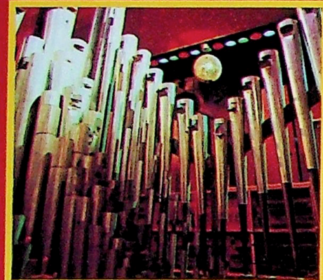
Foundation chamber front to back - English Post Horn, Tibia Clausa (large scale), Diaphonic Diapason, Tuba Mirabilis, Solo String, Tuba Mirabilis offset.
