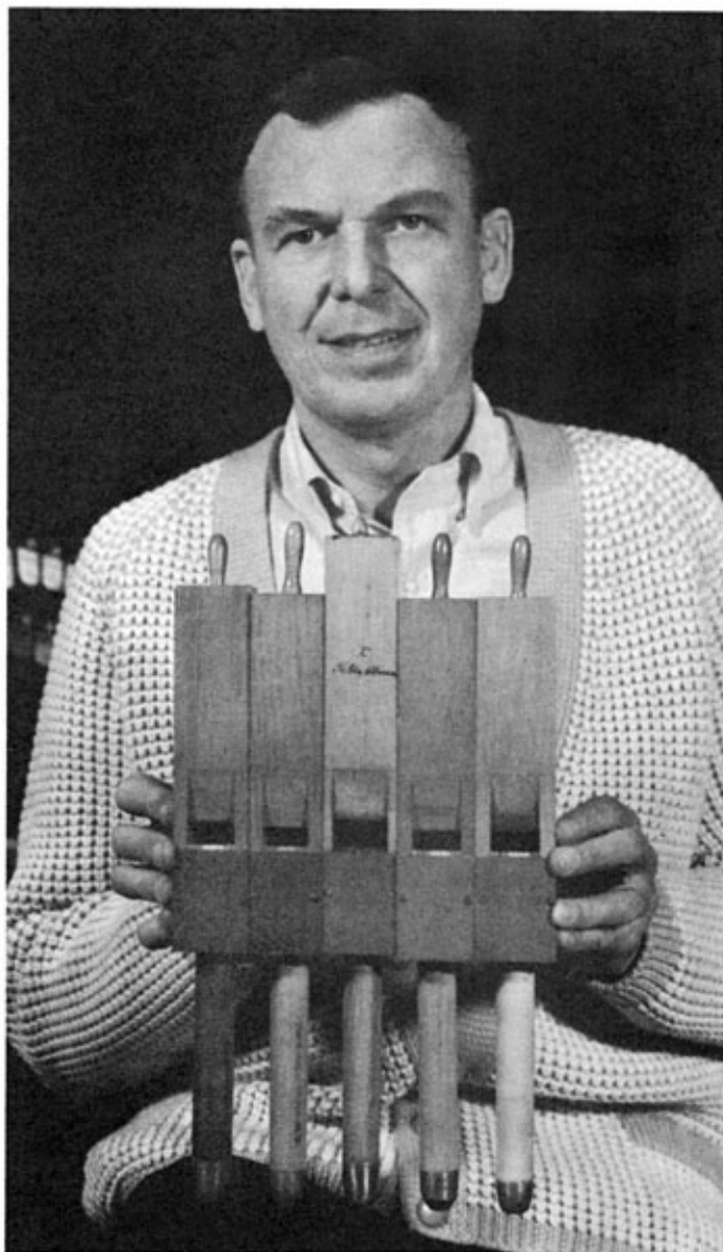
C ABOVE MIDDLE C IN QUINTUPLICATE - George holds C pipes from five Wurlitzer Tibias, all different. L to R, 1 has angular nicking, 2 is not leathered, 3 has an arched upper lip and no leather, 4 has very thin leather on its upper lip while 5's leather is extremely thick. George also has two Robert Morton Tibia sets
